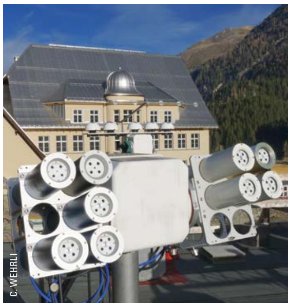
Several precision filter radiometers being calibrated against the WORCC triad of reference PFRs at Davos, Switzerland
