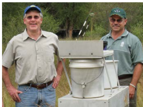
Typical collector used for precipitation chemistry sampling
