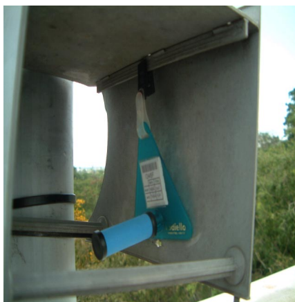
Figure 5. The passive sampler configuration used in this study.
