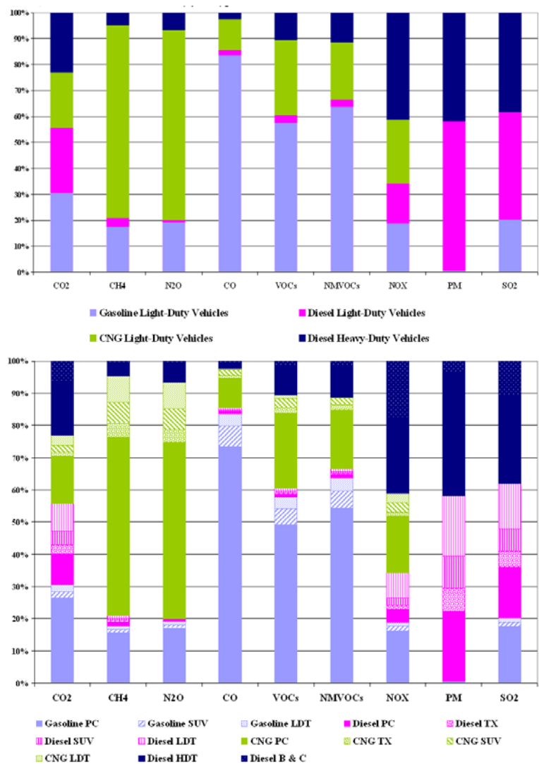
Figure 3. a) Emissions distribution by fuel type; b) Emissions distribution by vehicle category
